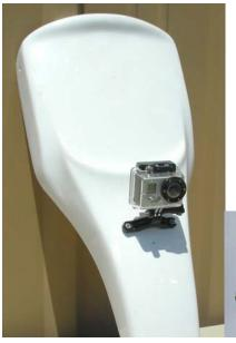
The mounting location is on the front panel. The installation kit must be fixed horizontally, in the middle of the panel, and between 300 mm (11.810") and 400 mm (15.748") from the upper edge.
